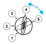
2. If the temperature is above  $-12^{\circ}$ C (10°F) and the engine does not start within five seconds on the first try, turn the key to OFF, wait ten seconds and try again.
